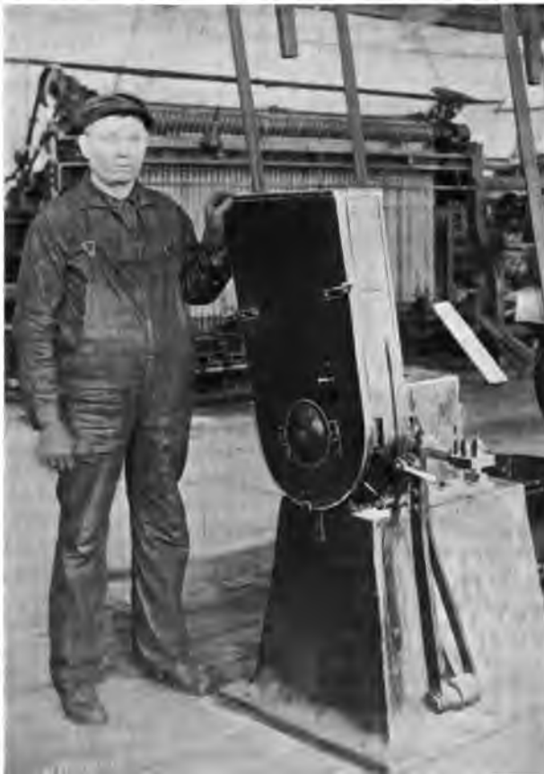
Fig. 3. Belt Guard. (American Steel and Wire Company, subsidiary of United States Steel Corporation.)
